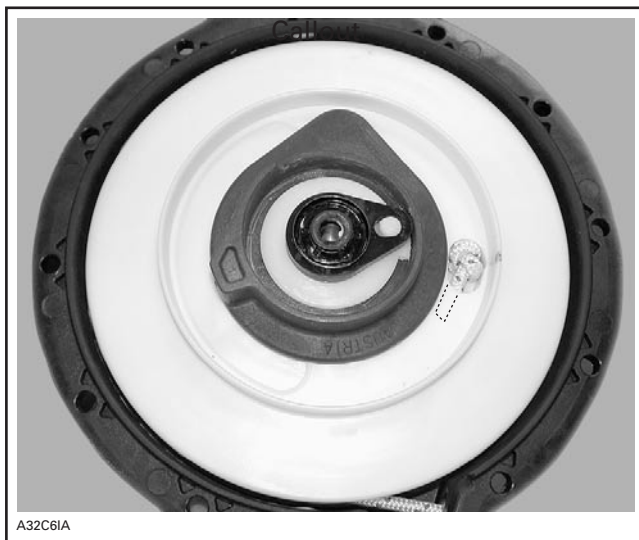
FREE PORTION INSERTED INTO SHEAVE
