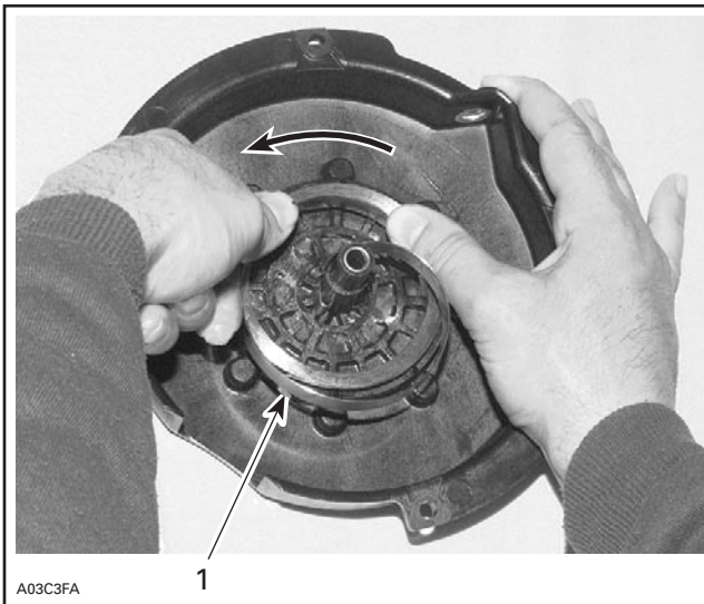
1. Outer end into guide notch
