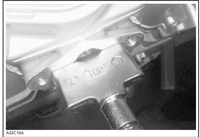
RAVE VALVE PARTIALLY REMOVED
