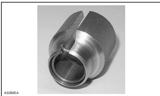
CIRCLIP READY TO BE INSTALLED ON PISTON
