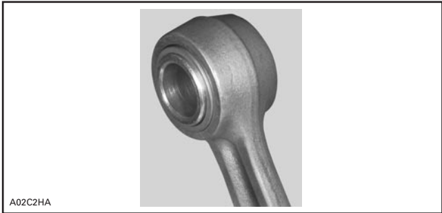
TYPICAL — CAGELESS BEARING AND SLEEVE INSTALLED
