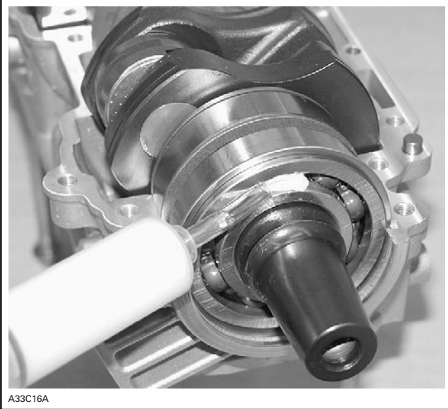
BALLS COATED WITH A SEAM OF GREASE
